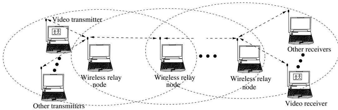
Fig. 3. Wireless ad hoc transmission scenario. The actual number of relay nodes depends on the simulation. Each dashed ellipse represents the coverage of the device in its center, thus each end-to-end transmission needs to traverse all relay nodes.
