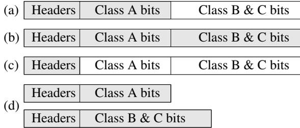
Fig. 2. Comparison of transmission schemes: proposed partial checksum (a), full checksum (b), header-only partial checksum (c) and UEP (d). Both MAC and IP/UDP/RTP protocol headers are always protected. The shaded area represents the checksum coverage.
