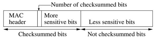
Fig. 1. Data-type 802.11 MAC frame structure modified for partial checksum.
