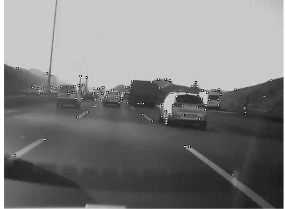
Fig. 2. Example of key points determined by the KLT feature tracker.
