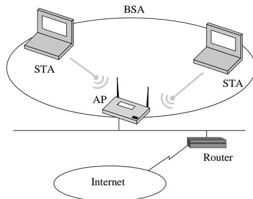
Fig. 1. 802.11-based network communications scenario.
