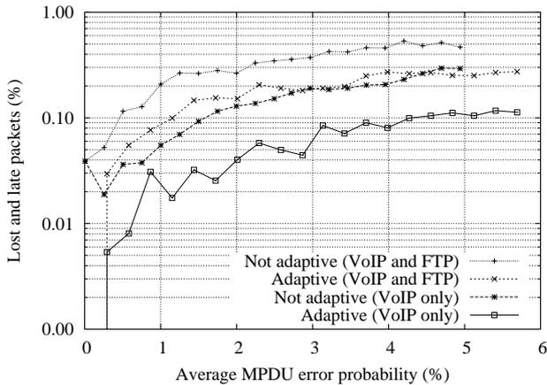
**Fig. 3.** Lost and late speech packets as a function of the average MPDU error probability; adaptive vs. not-adaptive technique, with and without interfering FTP traffic.
