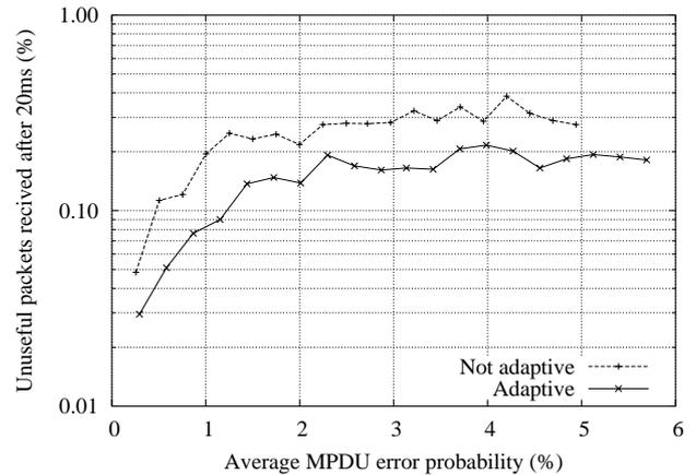
**Fig. 4.** Packet discarded at the receiver because of their late arrival (delay larger than 20 ms) as a function of the average MPDU error probability. Adaptive vs. not-adaptive technique.
