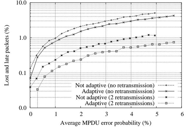
**Fig. 2.** Lost and late speech packets as a function of the average MPDU error probability; adaptive vs. not-adaptive technique, maximum number of retransmissions set to zero and two.
