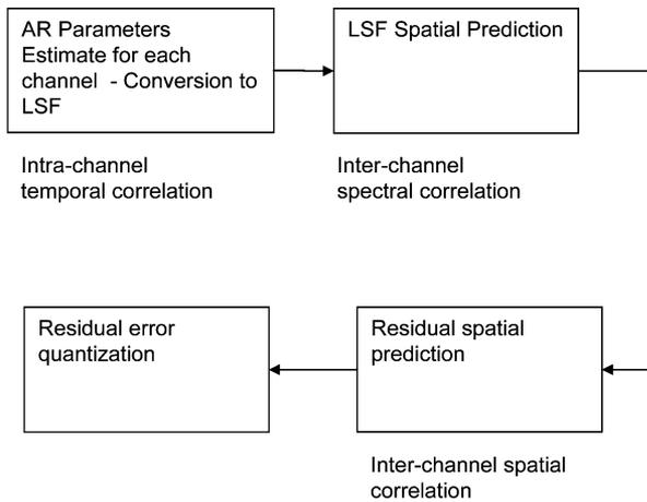
Fig. 1. Block diagram of the proposed technique. The AR model parameters are estimated for each channel, then the interchannel dependency is removed between both the LSF parameters and the prediction residual data using past coded data from spatially adjacent signals. The resulting residual error signal is vectorially quantized by means of analysis-by-synthesis. See text for details.
