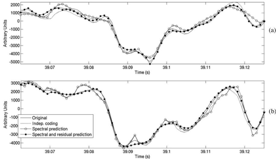
Fig. 2. Portion of two adjacent EMG signals from the same multichannel recording. The original signal, and the reconstruction from independent coding, spectral prediction, and the proposed technique are depicted. Compression ratio for independent coding was set to 89.6%, whereas 91% was set for both spectral prediction and the proposed technique.
